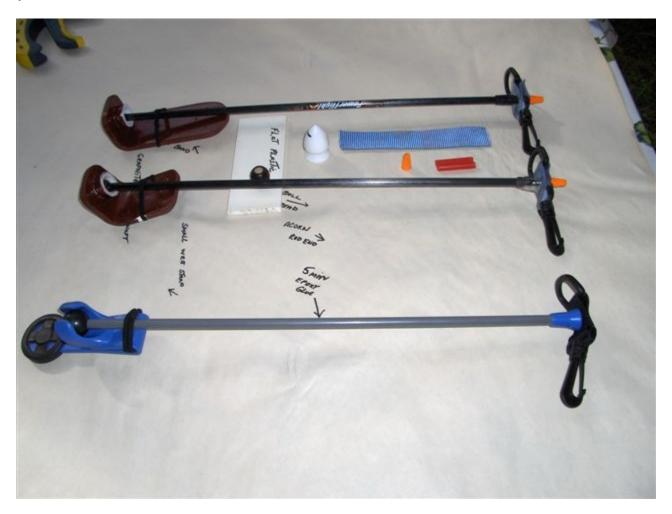
What is the idea of a Hip-mount? Quite simply it is useful in minimizing the weight on the arm carrying the detector without restricting the side to side motion common with the use of a metal detector.
