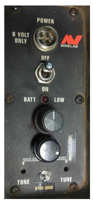
This is the frequency control. Middle is the standard 2100 frequency, the bottom is a faster frequency which will be good for smaller shallow targets and finally Upwards is a slower frequency for deep larger targets.
